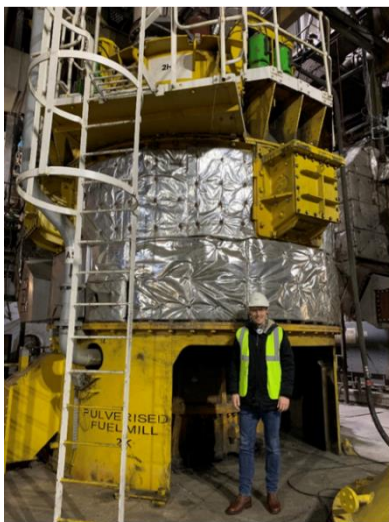
The machines pulverising the wood pellets to dust
