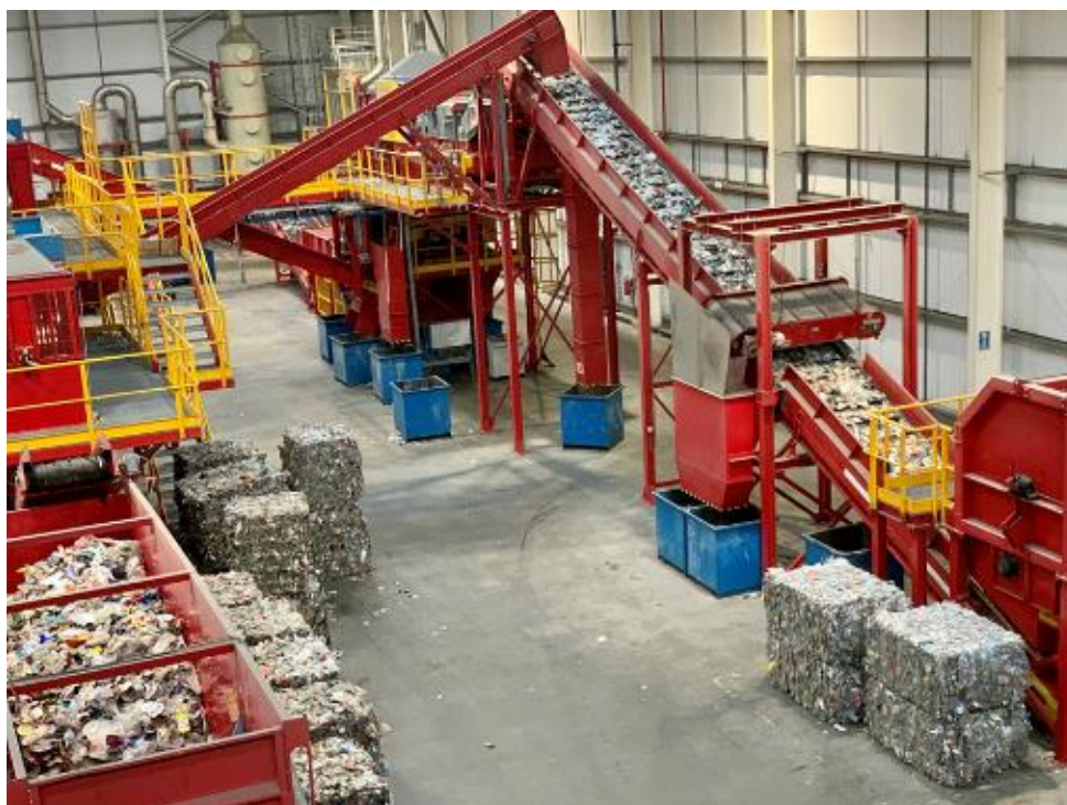
The bales are broken down and the items begin to move up a conveyor belt
