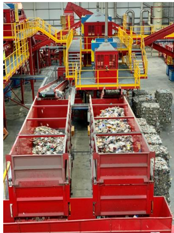
Labels, sleeves and other unwanted waste are collected in the large red bins
